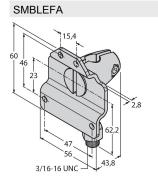
Mounting bracket, rotatable, stainless steel, for sensors of the LE250/550 series
