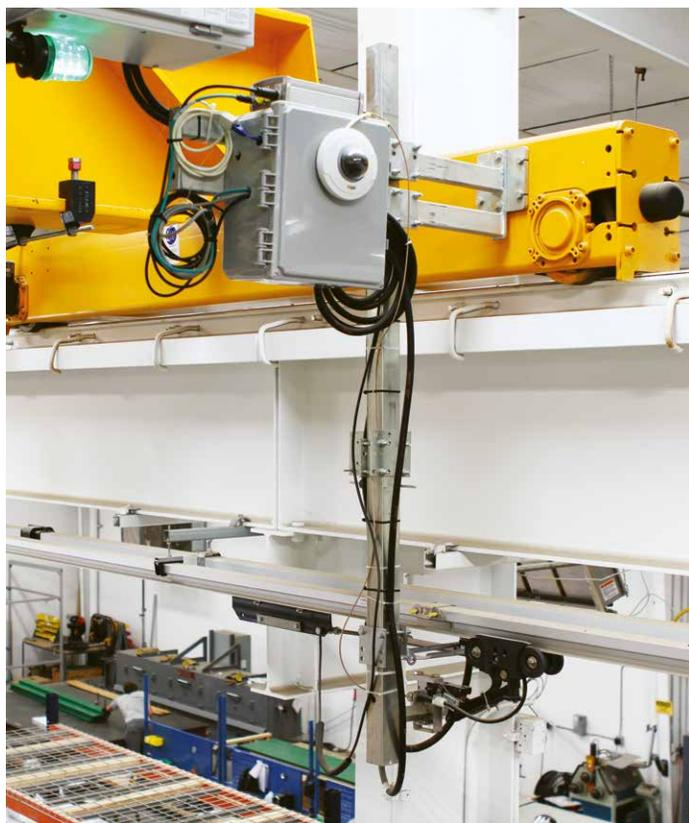
KBH, APOS® and SMGX installations for automating the crane in an industrial warehouse
