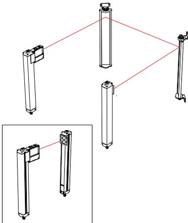
Figure 14. Optical alignment using the LAT-1-LP
