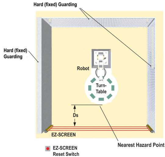
Figure 3. Safety distance and hard (fixed) guarding
