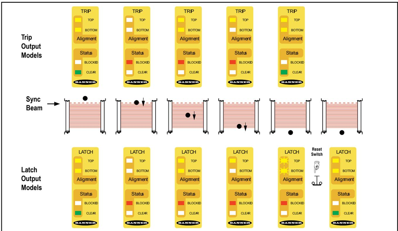
Figure 21. Status Indicator behavior during the trip test
