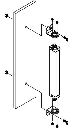
Figure 10. Emitter and Receiver End-Cap Mounting Brackets
