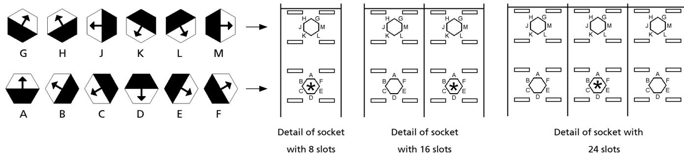
\*: receptacle to be left free in the event that the relay is fitted with an antirotation pin.
