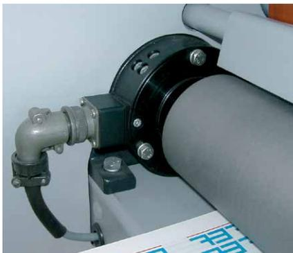
Flange load cell PD 21 on re-rolling machine
