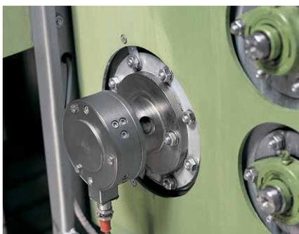
Flange load cell PD 23 on washing machine
