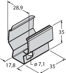
Snap bracket for mounting WLS28 work lights
