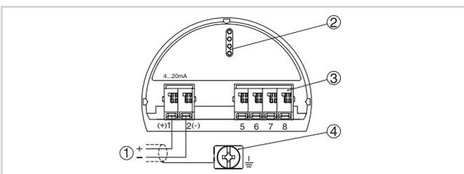
Electronics and connection compartment, single chamber housing
