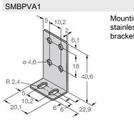
3056884 Mounting bracket, for PVA and PVD, stainless steel; set consisting of two brackets and screws
