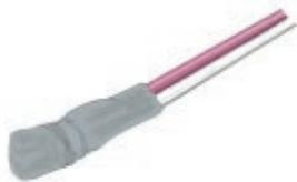
Platinum resistance temperature sensor on ceramic substrate protected by a heat-shrinkable sleeve and with PTFE isolated stranded wire. The TF101K version can be installed in motor or transformer windings. When build-in into windings do not pressure the sensor element. Precautions should be taken to protect sensor and extension leads against push and pull forces. Thermal response time  $T_{0,9}$  in the air 100 s, in water 19 s.
