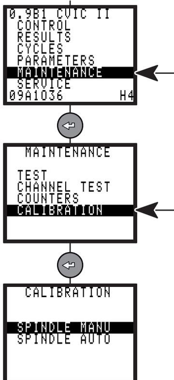
The calibration procedure is recommended to compensate for any possible drift of the tool torque or after each change of tool element.
