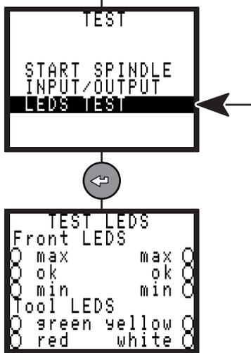
This menu allows for testing the LEDs located on the front side of the CVIC and for testing the LEDs on the tool.
