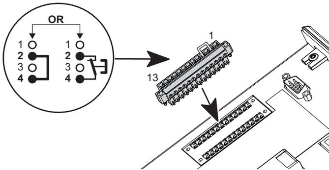
The opening of the STOP contact disables the power circuit. Note that it is recommended to wire the STOP when using handheld tools, but that it is absolutely necessary for fixed tools.
