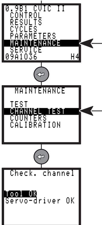
This menu is used to test the operation of the controller and tool. There is a sequence of two tests:
