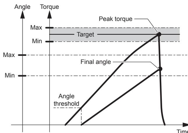
The start of the angle threshold counting should be within the linear area of the torque increase.
