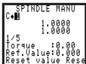
This menu is used to calculate and to apply a torque correction coefficient to the torque value of the selected cycle.
