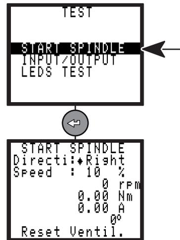
The START SPINDLE menu allows you to check the correct operation of the tool.
