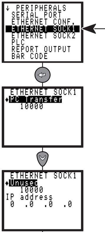
The ethernet socket 1 is used for the following function:
