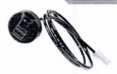
The T/LL200 series is designed for use in vented tanks requiring continuous level measurement of their contents and provides a factory set linear\* voltage or 4-20 mA output suitable for connecting into a PLC or process related applications. (The T/LL200 is not a loop powered sensor).
