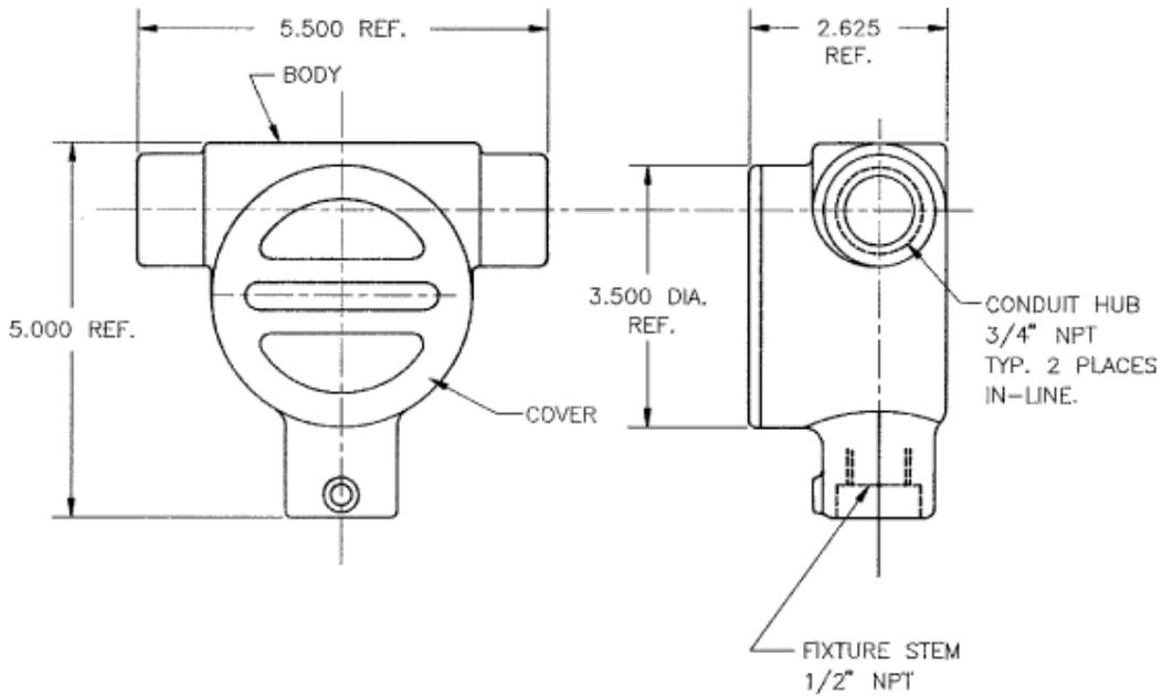
Figure 4. Optional Explosion Proof Enclosure, P/N 06-116317-001
