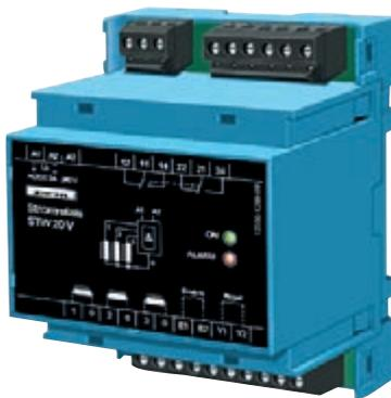
The current relay STW20V monitors the current in up to 3 lines with current transformers STWA 1 (AND circuit). If there is a current in all 3 monitored lines, the relay (2 change-over contacts) picks up. If there is no current in at least one of the lines, the relay releases.
