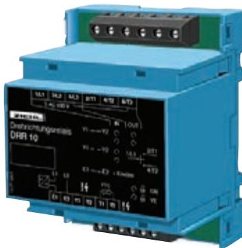
Phase-sequence relays DRR10 measure the sequence of the phases when being switched on and switch - if necessary - the rotation of the field by changing 2 phases.
