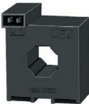
The ASS500/5 plug-in-current-voltage transformer is a measuring transformer with high linearity for currents up to AC 500 A and an output signal of 5 mV per ampere. Its maximum error is 1% of the measured value. The instrument is simply plugged onto the current-carrying conductor.
