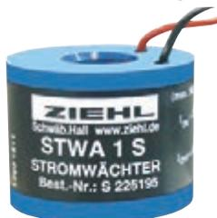
The STWA1S has an integrated electronic with transistor-output. The switching point is 2A. Above app. 2 A the output transistor is switched on (LOW), below app. 1.5 A it is off (HIGH).
