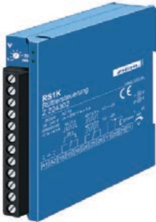
The vibrator control RS1K is a compact multiple time relay for triggering of vibrators in suction plants. In order to be able to operate suction plants at an optimum, the filters which get clogged by sawdust, chips or dust, have to be dedusted by vibration from
