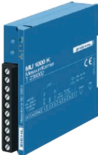
Universal-measuring-transducers MU1000K can measure signals Pt100 (RTD) and DC current (0/4-20 mA) and voltage (DC 0/2-10 V). Several measuring-ranges are pre-programmed. More can be easily scaled. Temperatures at sensors Pt 100 can be evaluated from -200 °C to + 800 °.
