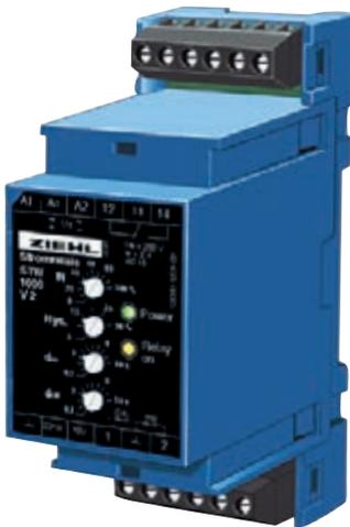
ZIEHL STW1000V2 current relays monitor standard signals from instrument transformers for compliance with a limit value. Units can be wired in series (current) or in parallel (voltage) to monitor multiple limits. Measurement inputs for 0/4-20 mA and 0-10 V, adjustable hysteresis and switching delays plus the selection facility to choose between the normally closed current and normally opened current principle for the relay make it a universal limit switch.
