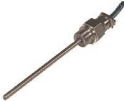
Platinum resistance temperature sensor built into steel tube V4A, 1/2 inch, suitable for installation in pipes. Thermal response time  $T_{0,9}$  in the air 255 s, in water 45 s.
