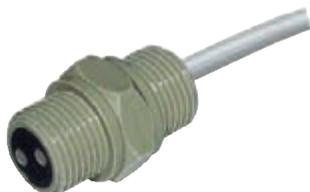
The electrode NE2 with its 1/2" thread can directly be screwed into the wall of a tank. The two electrodes (stainless steel V4A) are flush cast in a plastic housing (Polypropylen, PP) with cast resin. The electrode can be used in a temperature-range -5...105 °C and is pressure-resistant up to 6 bar. The ingrained cable with 2 strands, each 0,25 mm<sup>2</sup>, is 2000 mm long,  $\varnothing$  4 mm.
