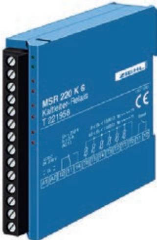
The MSR220K6 monitors up to 6 PTC-resistor sets with up to 6 PTCs each at the same time. If a temperature rise occurs in one set, the output relay releases and LEDs show the overheated sensor.
