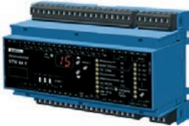
The current relay STW84V monitors up to 8 alternating current sets on current flow yes/no. The inputs can analyse signals of current transformers type STWA1 or of potential-free contacts. For controlling of great dedusting plants several relays can be combined.
