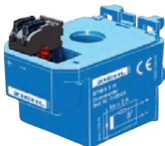
Current-transformers STWA1H can be fixed on a 35 mm DIN-rail or with 2 screws. The electrical connection is made via pluggable terminals. The cables are led vertical through the transformer (right angle to 35 mm-rail). The available diameter is 11 mm.
