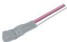
Platinum resistance temperature sensor on ceramic substrate protected by a heat-shrinkable sleeve and with PTFE isolated stranded wire. The TF101K version can be installed in motor or transformer windings. When build-in into windings do not pressure the sensor element. Precautions should be taken to protect sensor and extension leads against push and pull forces. Thermal response time  $T_{0,9}$  in the air 100 s, in water 19 s.
