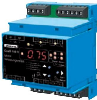
**Load monitors** protect motors in 1- or 3-phase mains from over- or underload. They are simply switched into the supply-line of the motor and monitor the phase angle between voltage and current and/or the true current.
