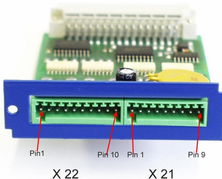
**Figure 32: E88: Position of the pin-and-socket connectors [X21] and [X22] at the front plate**
