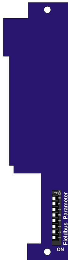
Figure 9: FBA module: Front view
