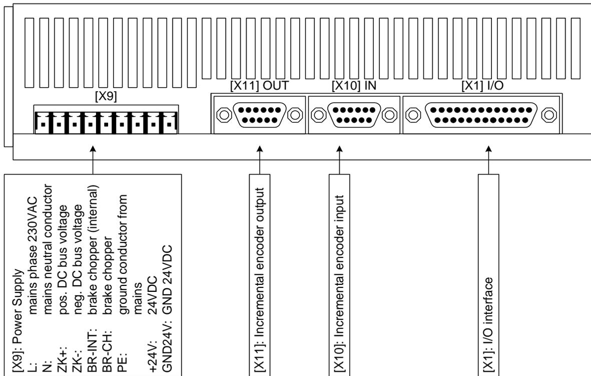
Figure 12: Servo positioning controller ARS 2102 FS: Top view
