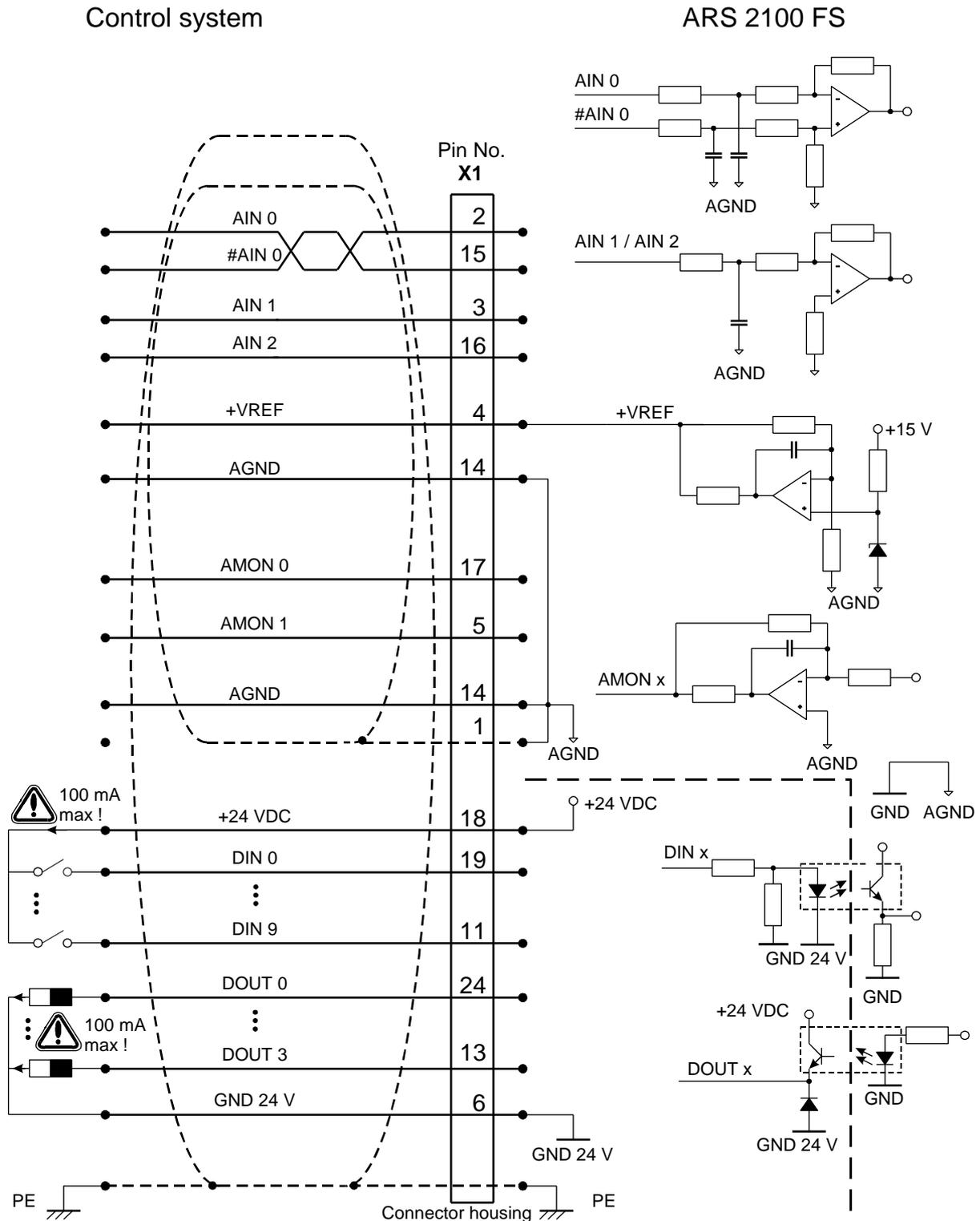
**Figure 20: Basic circuit diagram connector [X1]**
