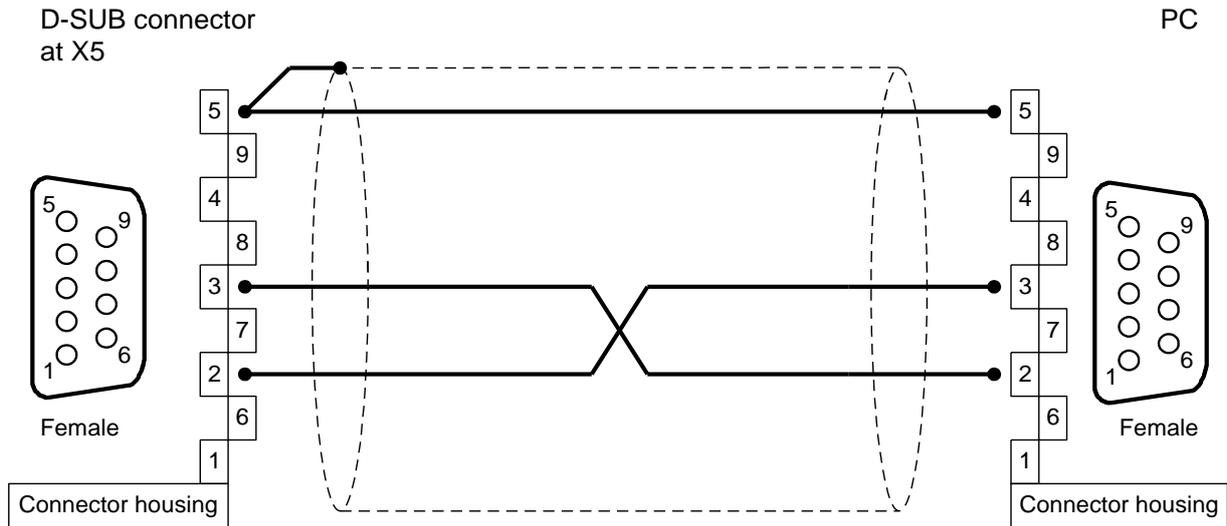
Figure 29: Pin assignment: RS232 null modem cable [X5]
