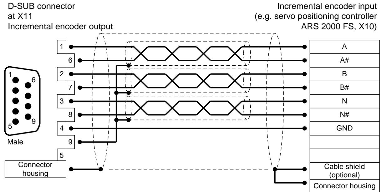
**Figure 26: Pin assignment: Incremental encoder output [X11]**
