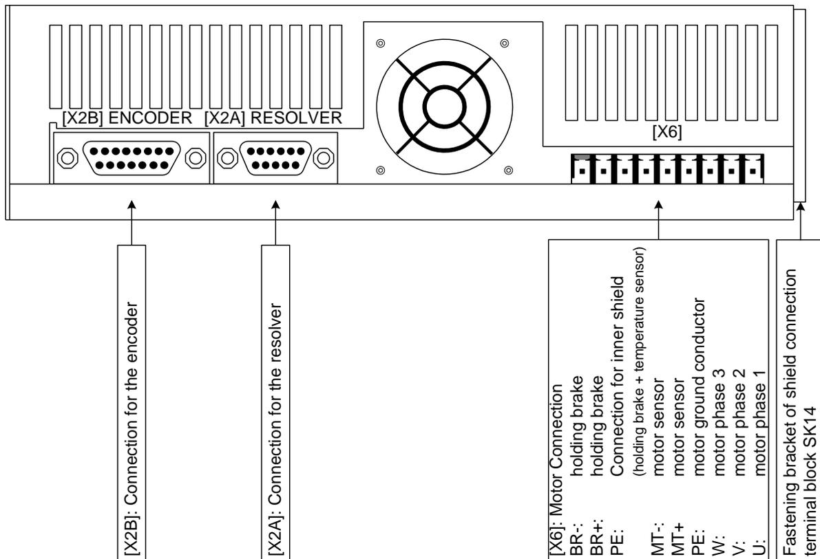
Figure 13: Servo positioning controller ARS 2102 FS: Bottom view
