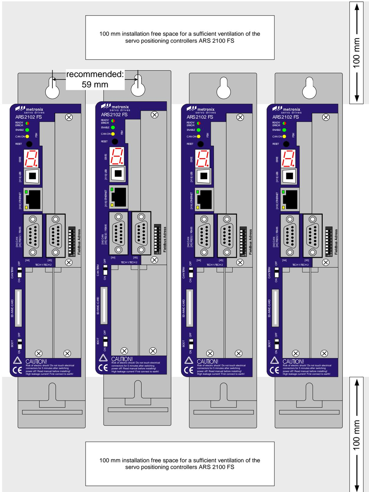
Figure 10: Servo positioning controller ARS 2100 FS: Installation space
