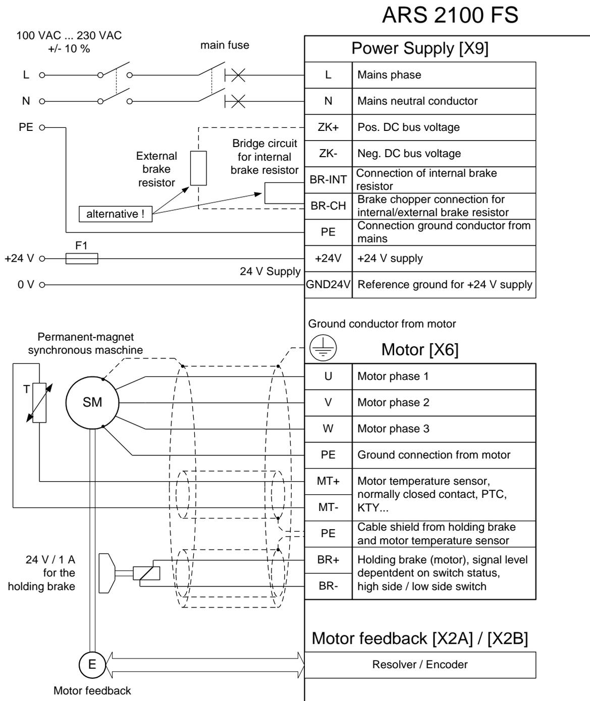
**Figure 15: Connection to power supply and motor**
