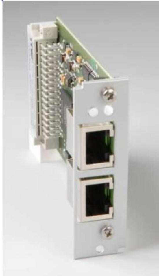
**Figure 36: EtherCAT module: Front view**
