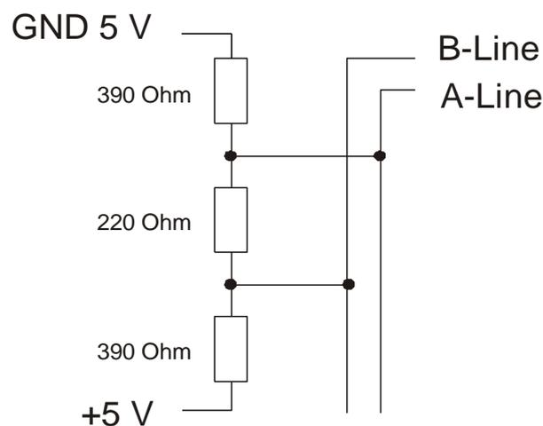
**Figure 34: PROFIBUS-DP interface: Connection with external terminating resistors**
