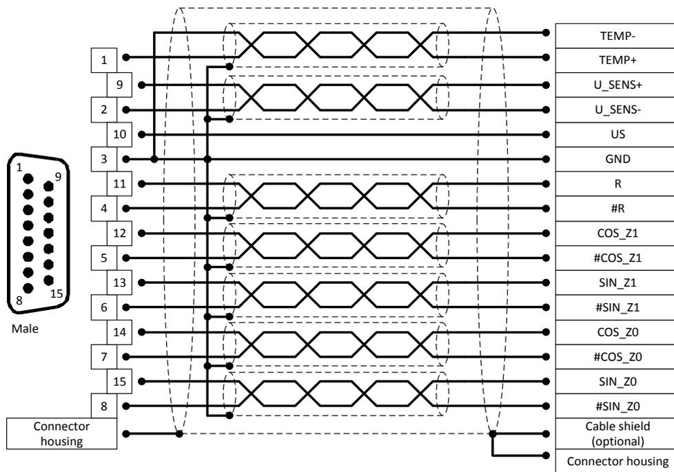
Figure 22: Pin assignment: Analog incremental encoder – optional [X2B]
