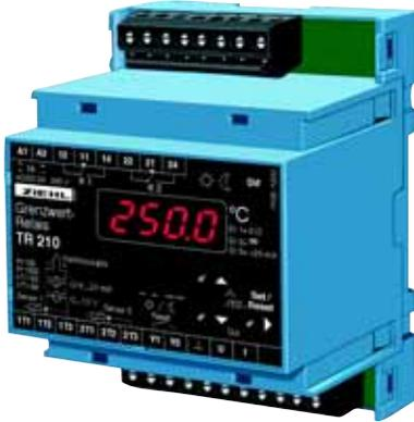
The limit value switch TR 210 monitors up to 2 measuring inputs for Pt 100 (RTD), Pt 1000, thermocouples, or standard-signals 0/4-20 mA, 0-10 V. The signals are monitored for up to 4 limits. The value of one or of both inputs can be read out at an analog output.
