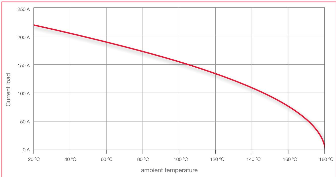
**Derating: Threshold value curves of screened copper high-voltage cables**
