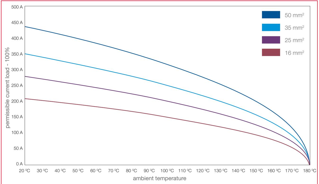
**Derating: Threshold value curves of screened aluminium high-voltage cables**
