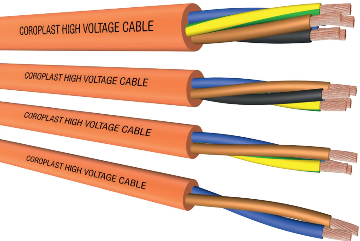
If required and upon proof of EMC suitability, unscreened high-voltage cables can be used as single-core cables in the so-called powertrain or as multi-core connection cables for vehicle-internal 230 volt plugs or other aggregates. The multi-core Coroplast high-voltage cables impress with their usability in the smallest construction spaces. Even in the event of extremely small bending radiuses, the original function of electrical safety remains in the vehicle across its entire lifespan.
