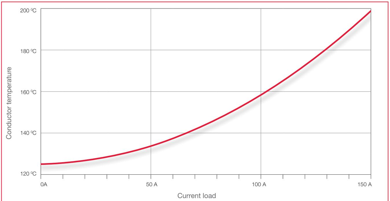
This type of derating curve can apply to only one environment temperature at a time. The curve shown above starts with an environment temperature of +125 °C.
