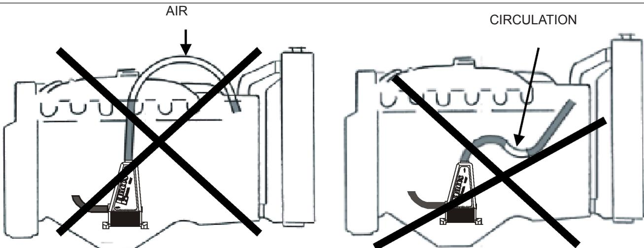
TO AVOID SIPHONS BEING PRODUCED; THERE SHOULD BE NO CURVES IN THE FLEXIBLE TUBES.
