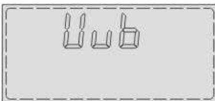
The top line of the display shows the codes for submenus and abbreviation for measurement values.
