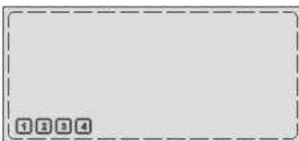
The bottom line of the display indicates which output relays are in active state.
