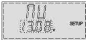
store the natural unbalance push the ► button. The second line of the display starts blinking and shows the actual measured value. To store the shown value push the ► button again. To set a new value for natural unbalance, just push the
