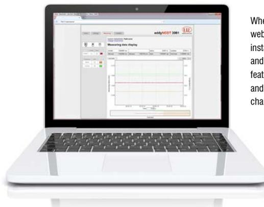
When connecting a PC via the Ethernet interface, a modern web interface can be accessed without any further installation and enables the parameterization of sensor and controller. The DT3061 controller provides enhanced features such as 5-point calibration, setting of switching and temperature outputs, as well as storage of multiple characteristic curves.
