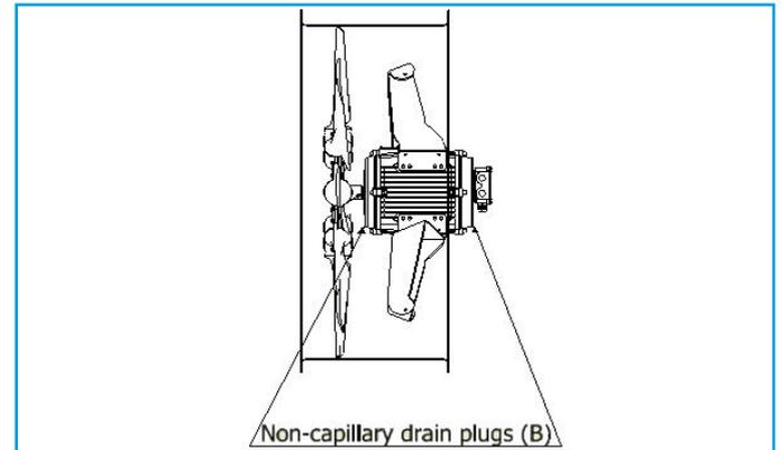
Figure 6. Horizontal mounted axial fans.
