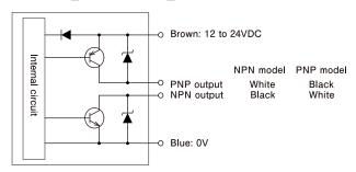
• Do not use the NPN and the PNP outputs simultaneously. Insulate unused output cable.
