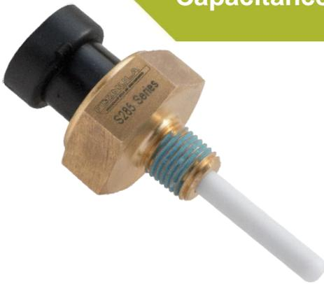
The **S285** is an active device designed to give an alarm signal if liquid falls below, or rises above, a preset level. It can be specified with a delay to eliminate false alarms due to turbulence.
