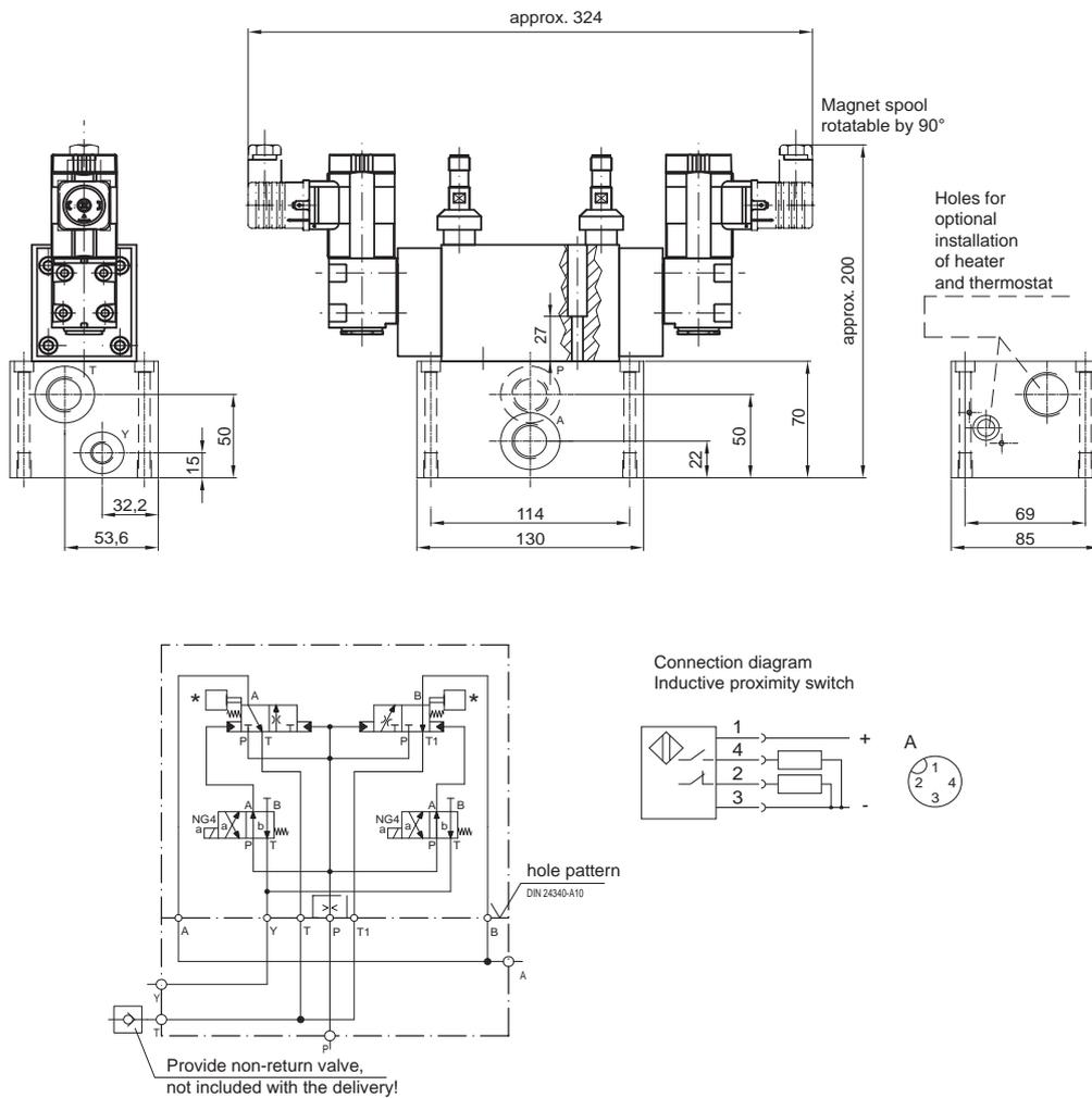
Fig. 1: Projection, hydraulic diagram
