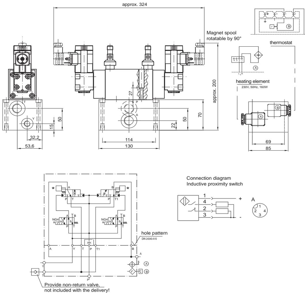
Fig. 2: Projection, hydraulic diagram
