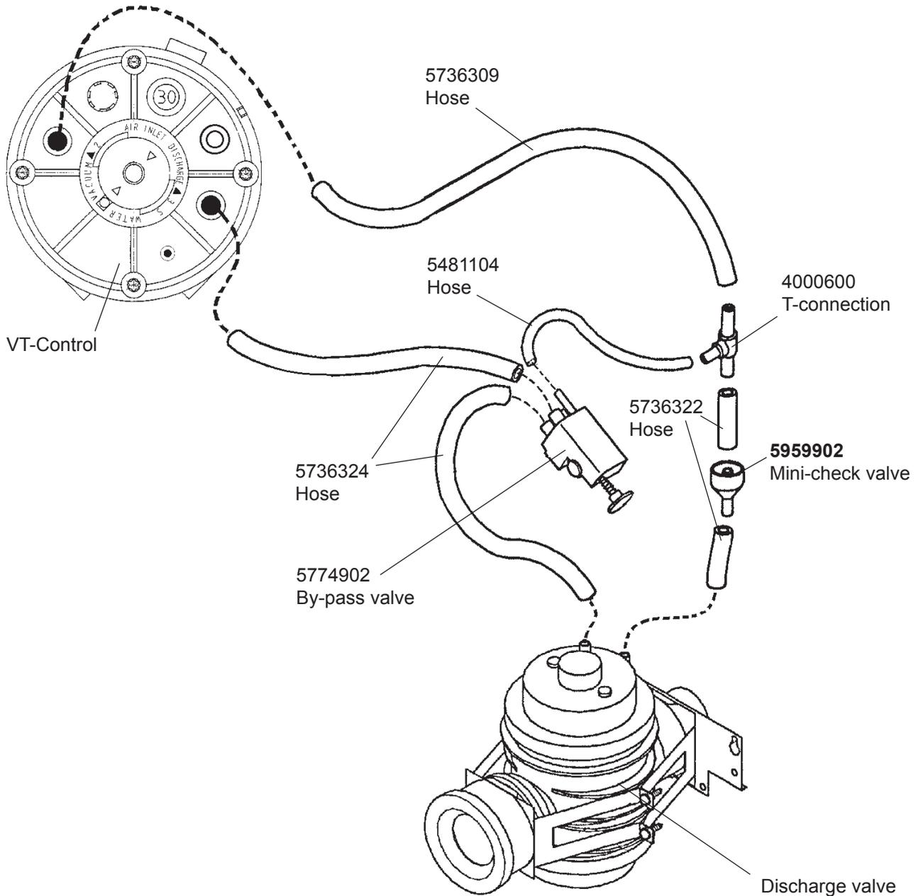
VT-Control and Discharge valve do not include in (P/N 5774903)
