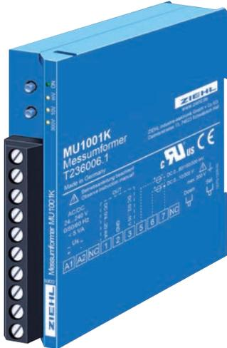
Universal Measuring-Transducers MU1001K can measure DC-signals up to 300 V. Inputs 60/150/300 mV are measuring DC current.
