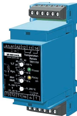
Temperature-Relays TR111V can be used as limit-switches or 2-point controllers with high repeat accuracy. 3 measuring-ranges, adjustable hysteresis and switching delay and the choice between operating- and closed-current principle of the relay make it a very universal device.
