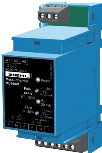
The MU100W measuring transducer converts the position of a potentiometer into a linear signal 0/4-20 mA respectively 0-10 V. Zero can be easily scaled 0...40 %, FullScale 60 ... 100 % of the range of the potentiometers by pressing a button.
