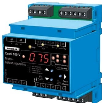
**Load monitors** protect motors in 1- or 3-phase mains from over- or underload. They are simply switched into the supply-line of the motor and monitor the phase angle between voltage and current and/or the true current.
