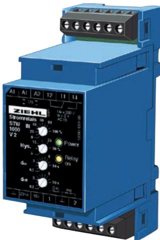
ZIEHL current-relays STW1000V2 monitor standard-signals from measuring transducers if a limit is exceeded. For monitoring of more than 1 signal, multiple relays can be connected in series (current) or in parallel (voltage). Measuring inputs for 0/4-20 mA and 0-10 V, adjustable hysteresis and switching delay and the choice between operating- and closed-current mode of the relay make it a very universal limit switch.
