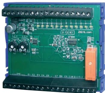
The current relay STW12 monitors the current flow yes/no of up to 12 alternating-current circuits. If there is an AC-current of  $\geq 1$  A through a connected transformer STWA 1, the according output transistor switches and the yellow LED lights up.
