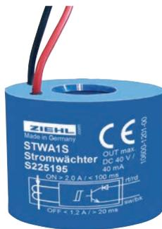
The STWA1S has an integrated electronic with transistor-output. The switching point is 2 A. Above app. 2 A the output transistor is switched on (LOW), below app. 1.5 A it is off (HIGH).
