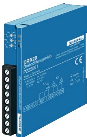
Phase-Sequence-Change Relays DRR20 measure the sequence of the phases and switch – if necessary the rotation of the field. At the output (connect relays K1 and K2 in series in this application) two contactors are connected. The contactor at the normally-open contact of K2 switches the phases 1:1 without changing them, the second (at normally-closed contact) changes 2 phases.
