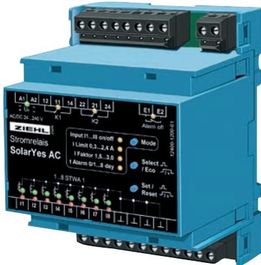
The SolarYes monitors outputs of inverters in PV-systems. Its output-relays (2 potential-free contacts) switch, when there has been no current during the last 24 hours in one of up to 8 monitored lines. Thus the failure of an inverter or a fuse is detected and reported. The operator can initiate repair immediately and saves downtime.
