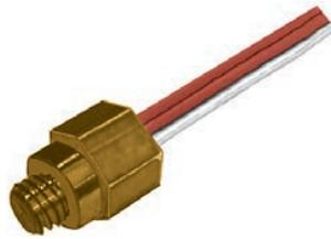
Platinum resistance temperature sensor on ceramic substrate built into a M6 brass threaded bush, especially suitable for being screwed into metal, e.g. for monitoring temperature of heat sinks or heating plates. Please note that there will be a measuring error due to the design, as the sensor can lose heat via the connection strand.
