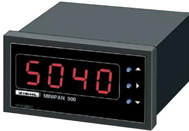
With its 4 digit, 14 mm high display, Digital Panelmeters of MINIPAN 300-series allow the accurate display of different values in the range -1999 ... +9999. Only 3 designs cover the measuring of DC voltage and current, AC voltage and current and temperature with Pt 100-sensors (RTD).
