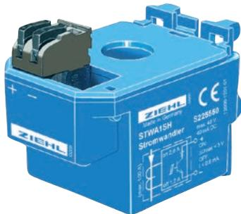
The STWA1SH has an integrated electronic with transistor-output. The switching point is 2 A. Above app. 2 A the output transistor is switched on below app. 1.5 A it is off.
