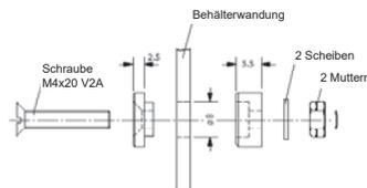
Insulated screw-in electrodes for mounting in walls of tanks. The electrodes are made of stainless steel (V2A), the material of the insulation is Teflon.
