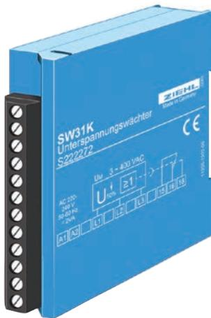
Undervoltage monitor for three-phase networks without N for monitoring on voltage failure. The voltage is being measured between phases and an artificial neutral point. At symmetrical decrease of the voltage to approx. 50% of the nominal value or in case of failure of a phase the integrated relay (1 change-over contact) releases with a delay of approx. 1s. With engines running on 2 phases, so much back voltage can be produced that the failure of a phase may be
