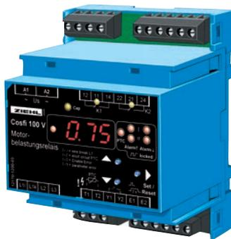
**Load monitors** protect motors in 1- or 3-phase mains from over- or underload. They are simply switched into the supply-line of the motor and monitor the phase angle between
