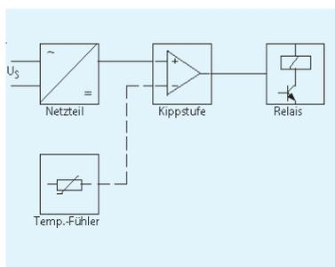
The electronics monitors the sensor-circuit with a continuous current. In the cold state the resistance is  $<250 \Omega$  per sensor and the relay signals o.k. The resistance of the sensors rise rapidly when reaching nominal response temperature (NRT). The relay switches at values
