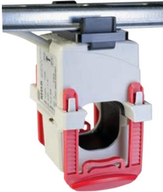
The split core current transformer KBR18S is especially suitable for being subsequently mounted in existing facilities. With its primary 60 A it matches perfectly the 63 A with which domestic connections are usually fused.
