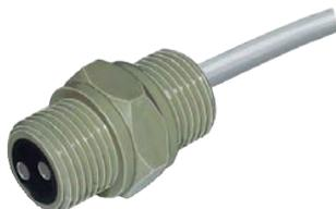
The electrode NE2 with its 1/2" thread can directly be screwed into the wall of a tank. The two electrodes (stainless steel V4A) are flush cast in a plastic housing (Polypropylen, PP) with cast resin. The electrode can be used in a temperature-range -5...105 °C and is pressure-resistant up to 6 bar. The ingrained cable with 2 strands, each 0,25 mm<sup>2</sup>, is 2000 mm long,  $\varnothing$  4 mm.
