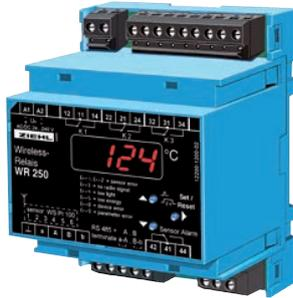
The Wireless-Relay WR250 is a receiver for up to 6 Wireless Temperature-Sensors WS Pt100. Up to 6 sensors transmit temperatures by radio. The WR250 displays and evaluates the temperatures.
