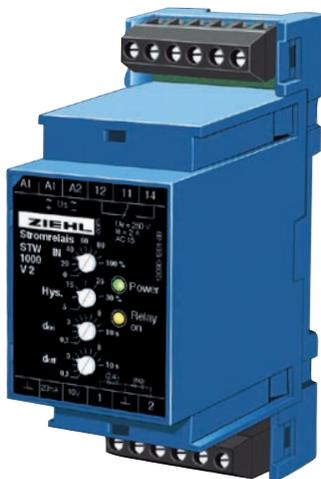
ZIEHL current-relays STW1000V2 monitor standard-signals from measuring transducers if a limit is exceeded. For monitoring of more than 1 signal, multiple relays can be connected in series (current) or in parallel (voltage).
