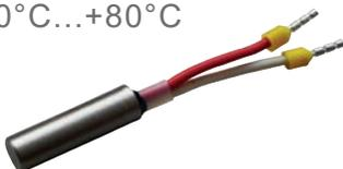
Sensors TF101U2 are encapsulated in a stainless-steel-shell V4A. They are suitable for measuring temperatures in fluids, at surfaces or for inside or outside applications. The protection class is IP 66. The version with PVC-insulated cable (3 x 0,25 mm<sup>2</sup> in one cable) can be easily wired. The maximum ambient temperature is 105 °C.
