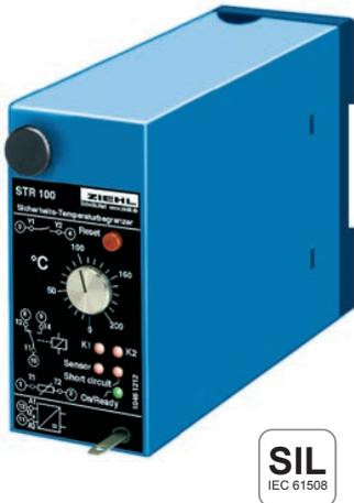
The electrical safety temperature limiting device type STR100, in connection with Pt100 sensors, monitors temperatures in applications for which monitoring with increased safety is required. Functioning corresponds to type 2BDK as per VDE 0631.
