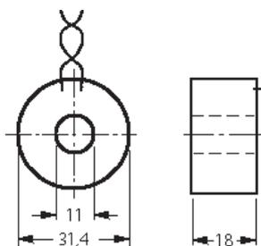
The STWA1 current transformer is made to match the STW current monitor. One current transformer is required for each line being monitored. The STWA1 consists of a climate-proven sealed-in coil with toroidal tape core. The connection cables are permanently fixed to the transformer and are 1 m in length. The level of the current to be monitored is limited to 100 A continuously, 300 A for max. 10s.
