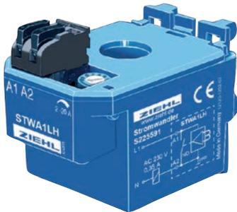
The electronic current transformer STWA1LH monitors alternating currents 2 ... 20 A. For lower currents, the monitored wire can be led multiple times through the transformer. Used in the secondary circuit of transformers (e.g. 100/5 A), it is possible to monitor higher currents.
