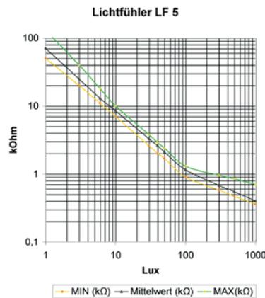
The light-sensor LF5 can be connected to the twilight-switches DS6 and DS6V. It is mounted in a hermetically sealed, weather-proof and uv-resistant plastic threadid pipe. The connection-cable is 1 m long.
