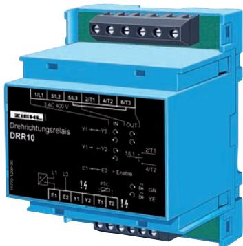
Phase-sequence relays DRR10 measure the sequence of the phases when being switched on and switch - if necessary - the rotation of the field by changing 2 phases.
