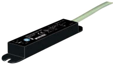
The current sensor S1 records the current in a cable with a hall-sensor. At currents of adjustable 5-30 A the transistor-outputs switch and report a current in the monitored cable.
