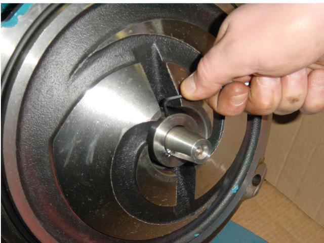
6) Tighten the socket head screw in the retaining ring carefully. The correct tightening torque is 7 Nm.
