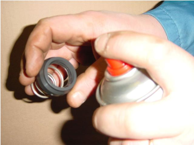
1) Lubricate the O-ring and the sealing surfaces with oil.
