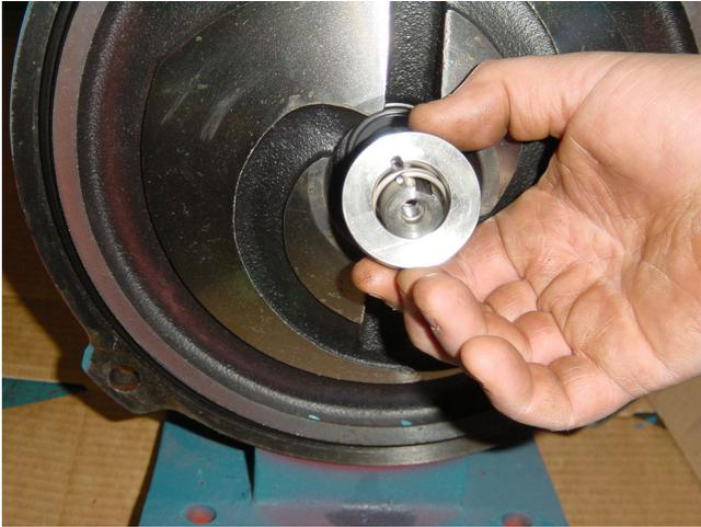
4) Be sure that the end of the spring will go into the groove in the retaining ring.
