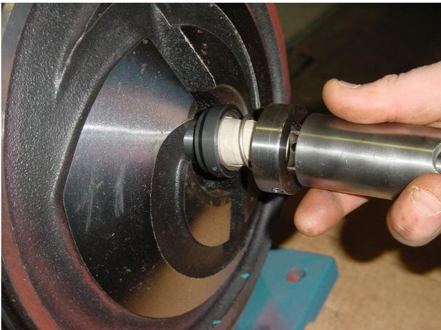
3) Push the rotating seal ring together with spring and retaining ring onto the shaft by using a suitable sleeve having inner diameter lightly bigger than 25 mm.
