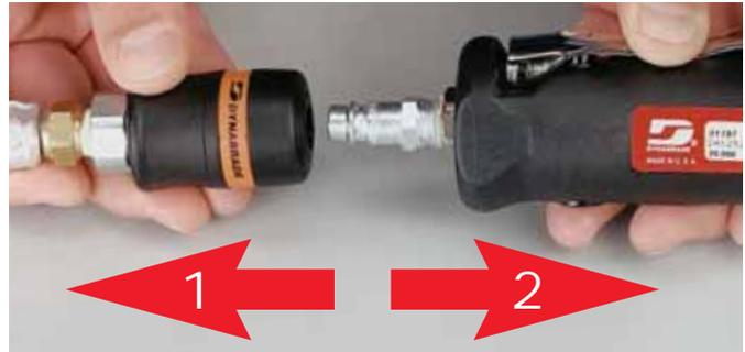
**Step One:** Pull back on the sleeve and the compressed air is vented.
